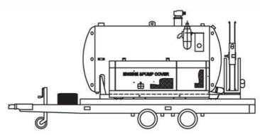
Vacuum tanker trailer designed with a capacity of 2200 litres Various water waste splits to suit requirements
