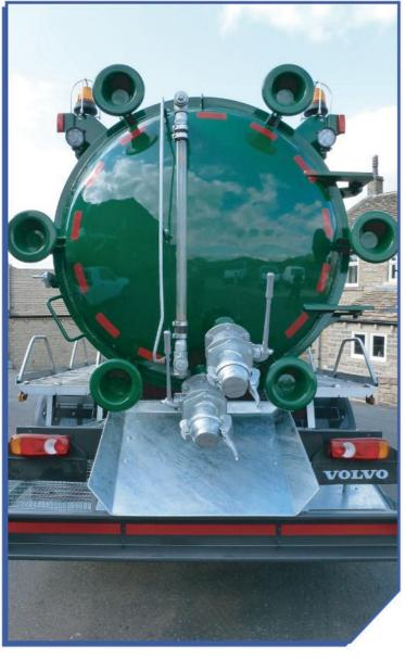
A Truck mounted 18 ton 2200 gallon pto operated welfare vacuum tank constructed from 6mm carbon steel with a capacity of 2000-gallon waste and 200-gallon fresh water (options available).
